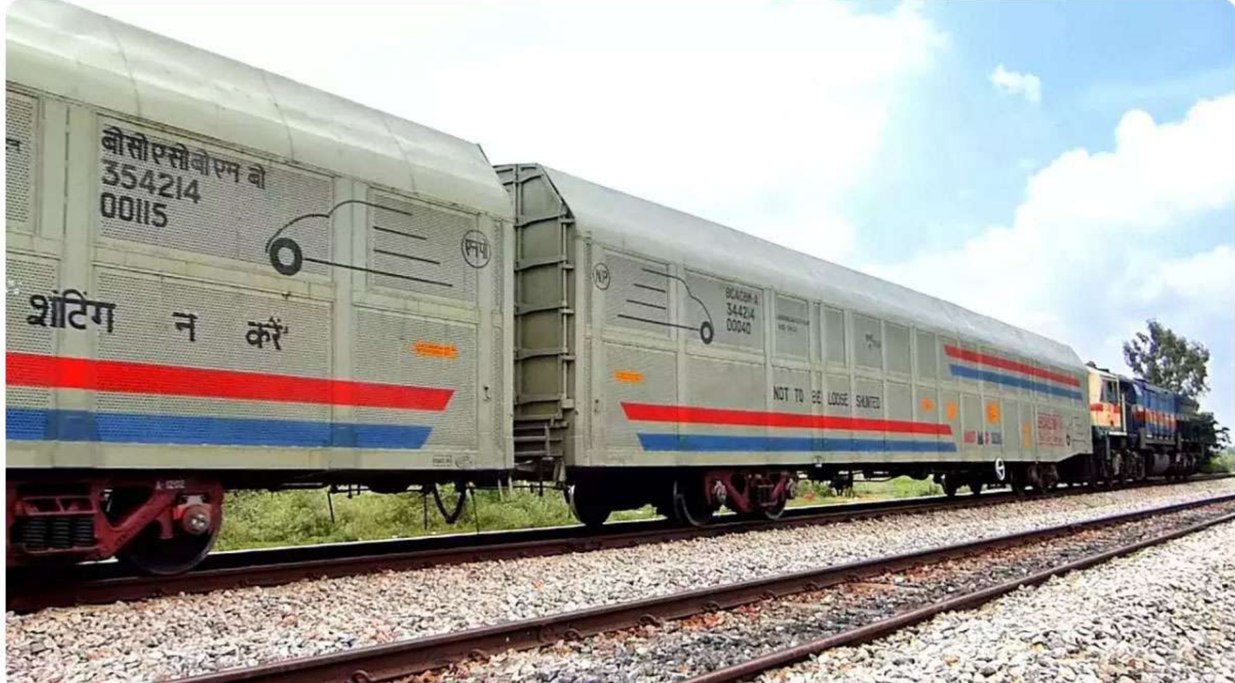
Currently, the NMG and the BCACBM Auto Loader wagons are used for transportation.
