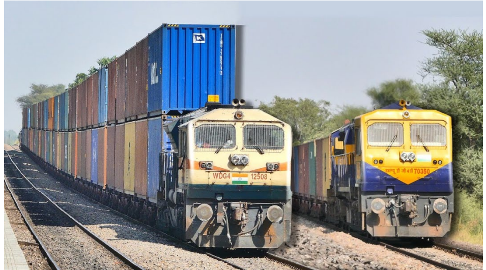
Fig. 1: Double stack train versus normal single container train
